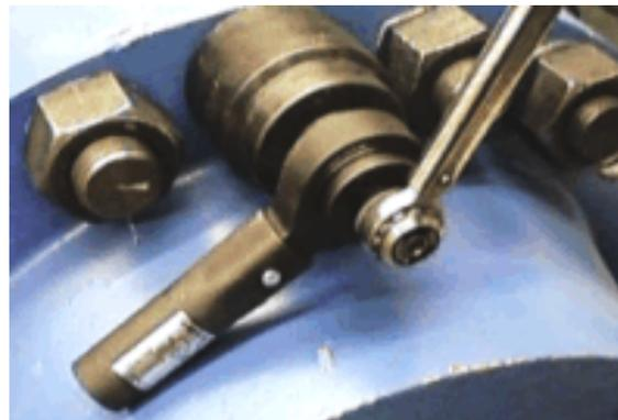
TORQTOOL Impact Socket used along with a TORQPLUS Torque Multiplier
